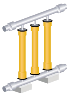
Equipment of overseas factory (Membrane filtration water purification system in this case)
